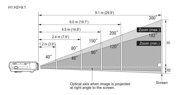
H1 and H2: H1 is the height of the screen from the intersection of optical axis and screen surface, and H2 is the height of the intersection when an image is projected at right angle to the screen.
